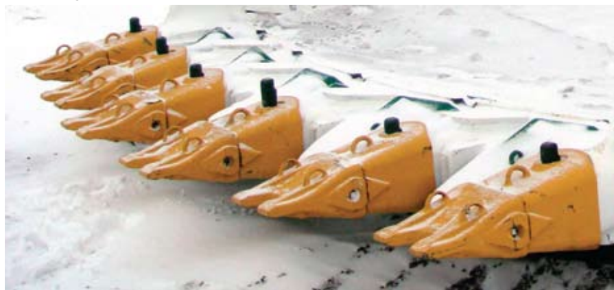
Caterpillar's LM series ground-engaging tools feature the CapSure tip retention design.
